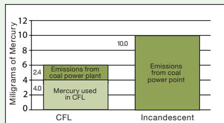
**Fig 6: Mercury Emissions by Light Source Over Year Life (Source: US EPA, June 2002)**
