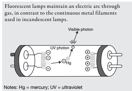
**Fig 4: Fluorescent lamp operation** (Source: E Source Lighting Atlas)
