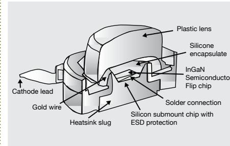
**Fig 8: LED Operation (Source: E Source Lighting Atlas)**
