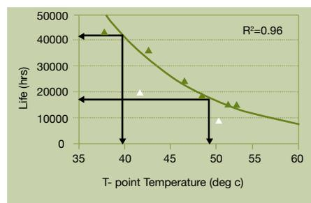
Fig 12: Effect of Junction Temperature on Life of LED Lamp (Source: Lighting Research Institute)
