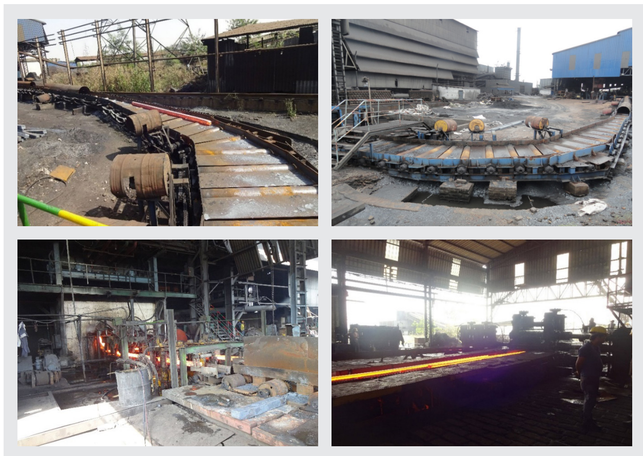
Figure 12: Photographs of direct charging of billets
